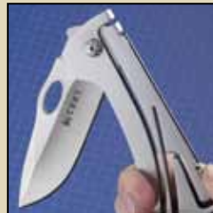
Press at the base of the spine to release the lock. A cam grind in the blade safely stops the blade at mid-point.
