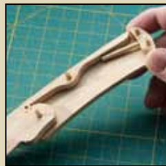
The bamboo spring and wooden locking bar are precision cut and can be easily assembled by press fit.
